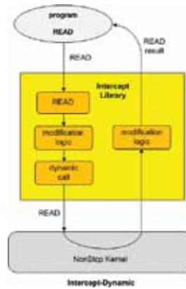
In the Intercept-Dynamic figure, a program invokes a system procedure READ and requests that data from the NonStop Kernel be sent to the program. Instead of the execution being transferred immediately to the system procedure READ, the intercept library captures the call via its own READ procedure, makes any call modifications that have been requested, then dynamically calls the system procedure READ. Dynamic calls are used to locate and navigate to the physical address of the system
