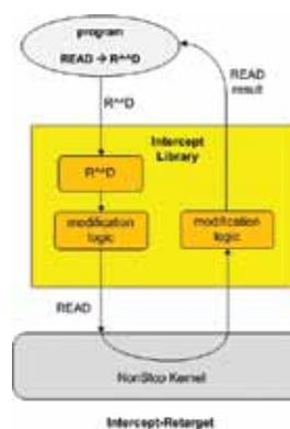
In the Intercept-Retarget figure, a program is “prepared” by assigning it an intercept library before any calls are executed. The program’s procedure calls are renamed to the intercept library’s equivalents. For example, calls to system procedure READ are changed to R^AD. Next, the prepared program and its linked intercept library are simultaneously executed. The intercept code, also named R^AD, is invoked instead of the system procedure READ. The intercept library linked into the
